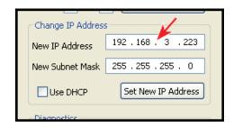
Please note that it is not a requirement to have a "sequential" IP address for the SX-48 units installed. You can even set up individual Subnet masks.
