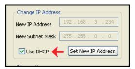
Simply click on the tick box <Use DHCP> ... then click on <Set New IP Address>. There is also a "direct" front panel feature on the SX48 to set this. Use a screwdriver (or similar tool) to press and hold the Setup button for 20 seconds followed by a 1 second key press. This will set the unit to DHCP mode.
